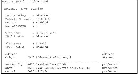
Figure 4-1. Example of Show IPv6 Command Output
